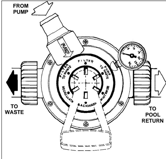
**FILTER:** Normal pool filtering position. May also be used when vacuuming the pool.
