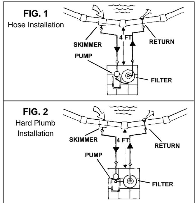
injury or damage to the filter system. Starting at least 12" from the pool wall, make two 3-4" deep trenches, one from the pool's skimmer toward the front of the pump and the other from the pool's return fitting toward the filter port located on the tank cover, marked "TO POOL". Be sure the hoses are routed so that water flow through them is not restricted.
